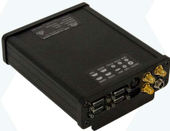
IVX (Back) - LMR and RF interfaces
